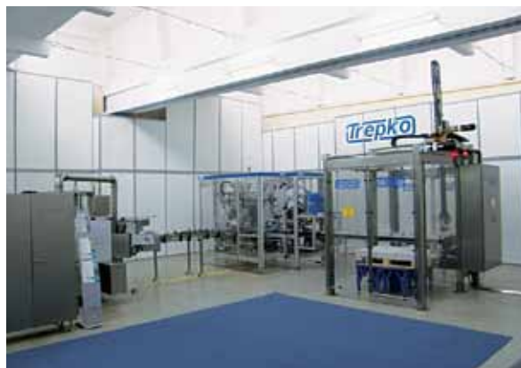
Complete line for bricks: PMG 4 (forming & wrapping machine), 710 (wrap-around cartoner), 740 (palletising robot).
