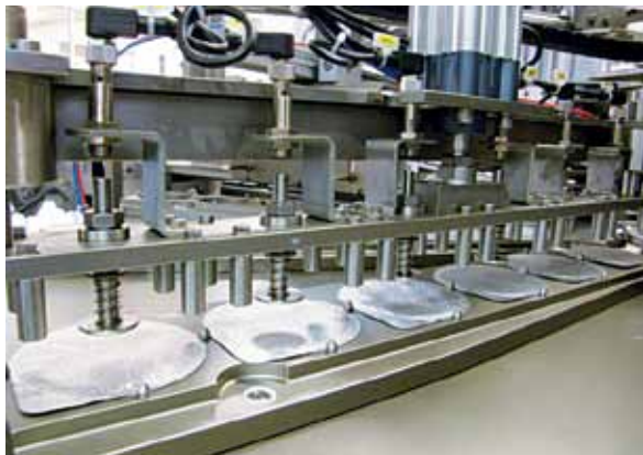
Seal-check station installed on a TREPKO 6-lane rotary machine (246 KSP).
