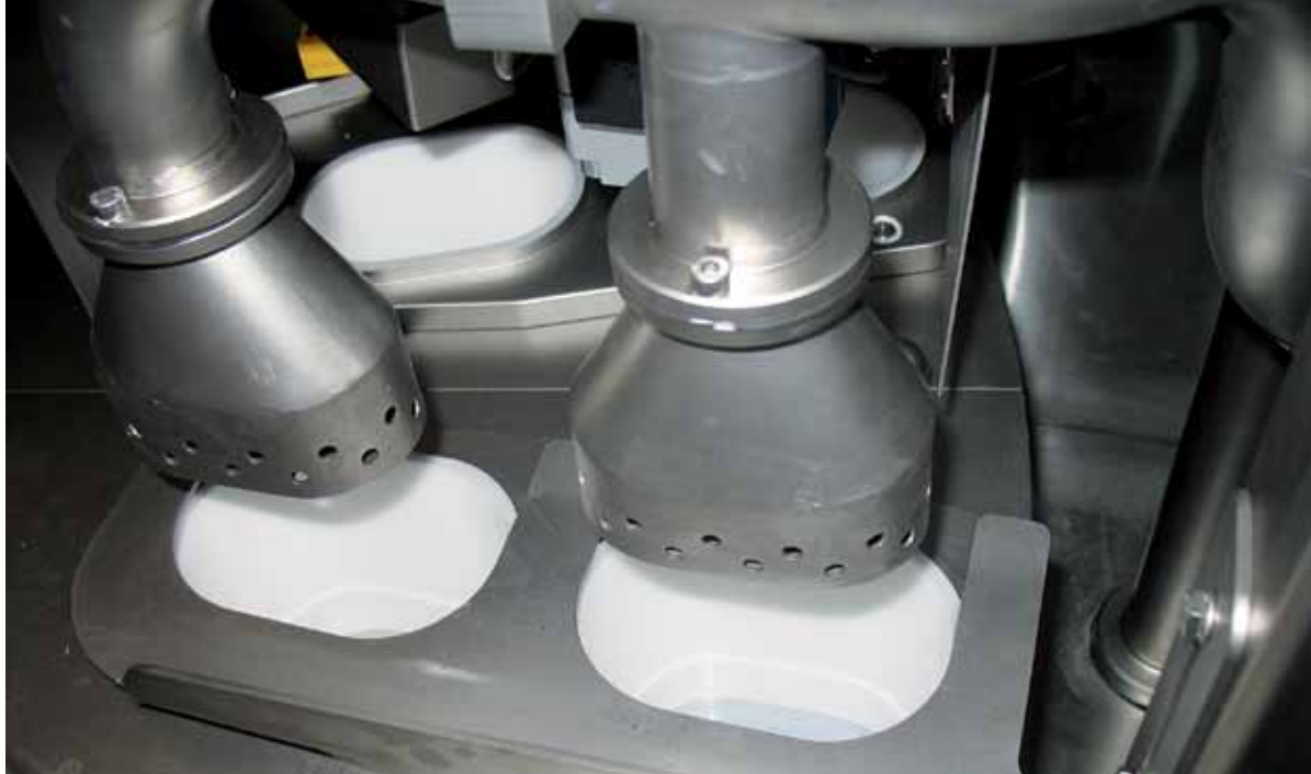
Vacuum cleaning of cups on a 232 KSP machine.
