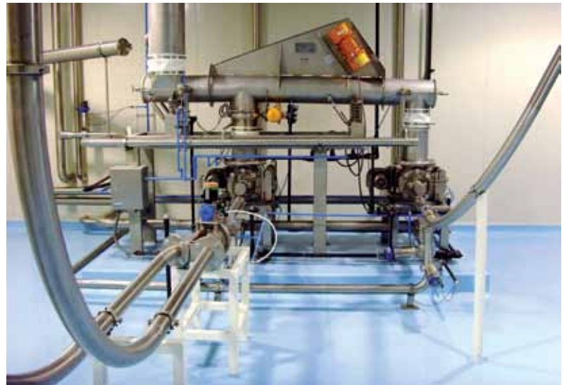
Reversible vibration Conveyors TRS with two outlets for babyfood.
