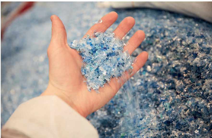
SKY-LIGHT manufacture rPET food packaging with up to 100% recycled plastic. One of the sources are shredded and recycled plastic bottles.
