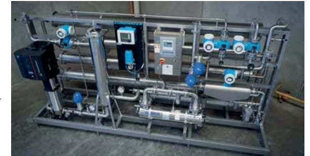
EUROWATER custom-made reverse osmosis unit in sanitary design for Danone Ukraine.
