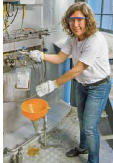
Laila Bleeg Smidt, Laboratory Technician, VitaLys I/S, removes a ferment sample from a Keofitt aseptic sampling bag.
