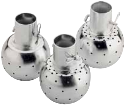
Image 1: Static spray balls use the low impact and high flow of cleaning media combined with the force of gravity to clean the tank. (Image: Alfa Laval LKRK Static Spray Balls).
