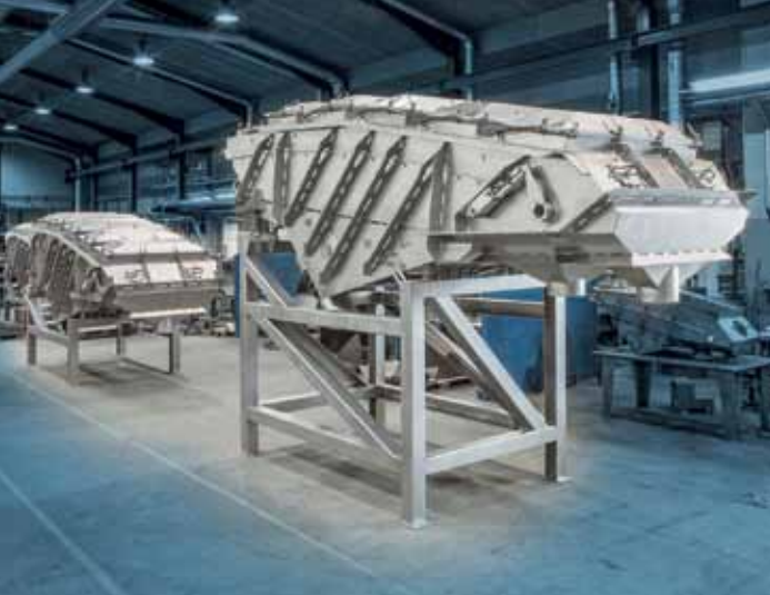
Picture 1: SRS 10 Vibration Sifter - 8 m 2 for baby food (dry cleaning).
