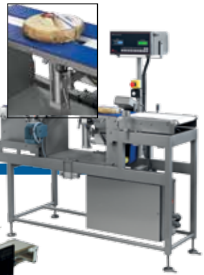
Figure 2: MID type approved check weigher.
