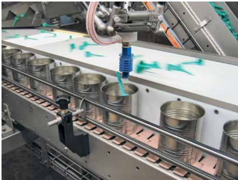
Infant formulas are booming, and a couple of years ago Jorgensen constructed the first of a line of advanced robotic systems for placing portioning scoops in canned infant formulas.
