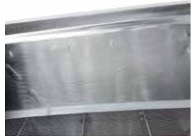
SRS vibration sifter, interior polish surface R_a < 0.8 .
